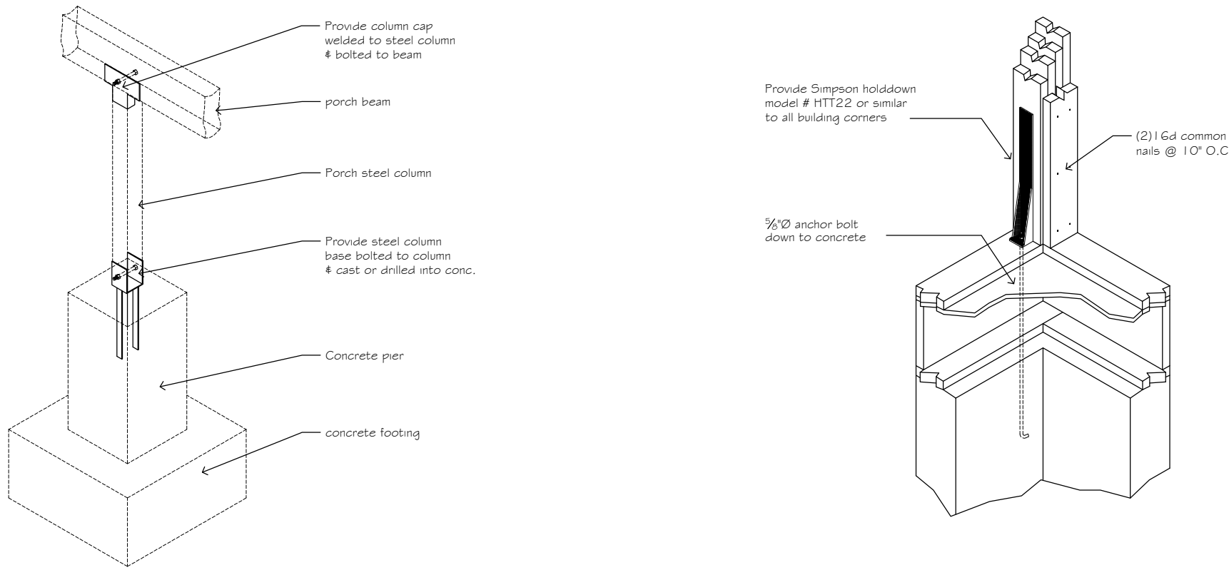
typical wood column & beam anchor detail not to scale typical corner holdown not to scale
